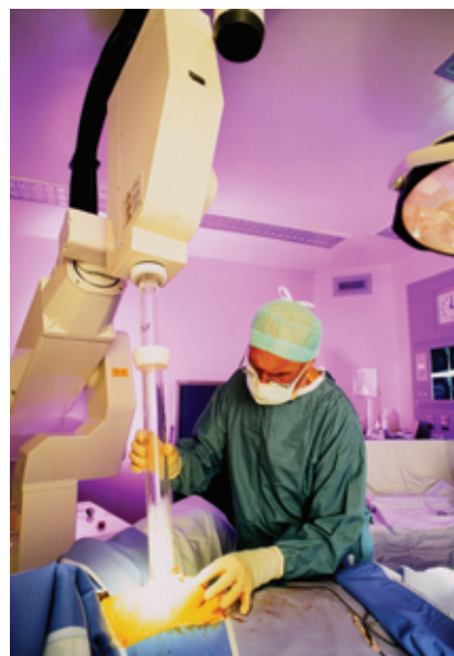
Figure 2: The Linac used for Electron Intra-operative Therapy (ELIOT) and ELIOT Applicator in Position
