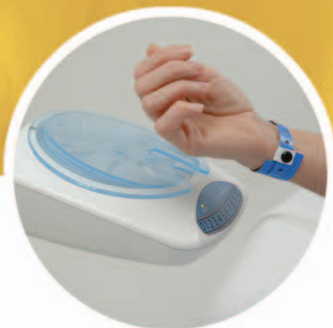
Patient Waves RFID Wristband Across the Faceplate to Activate the MOD.
